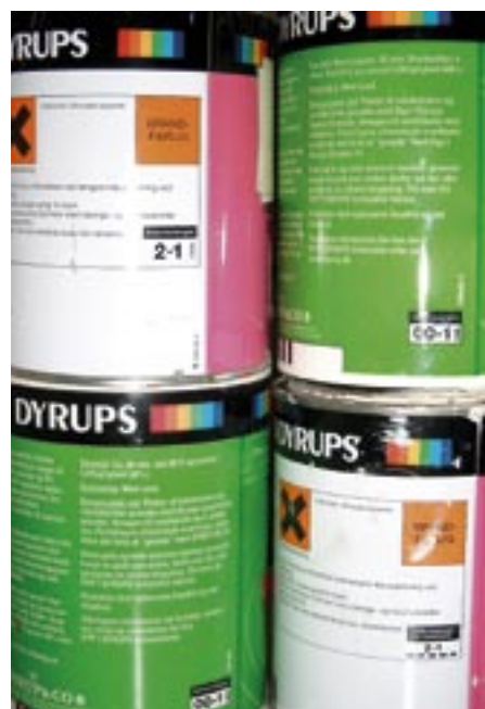
Figure 3 Paint product labelled with a MAL-code. The figure before the hyphen indicates the security measures to be taken after inhalation, whereas the figure after the hyphen indicates the security measures to be taken after having consumed the product or after skin has been in direct contact with the product. A low figure indicates low risks; high figure indicates high risks.
